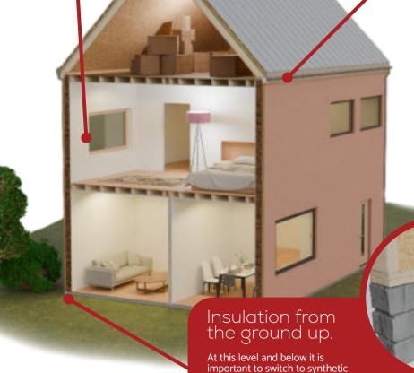
insulations that are not susceptible to moisture. The plinth area is insulated with
